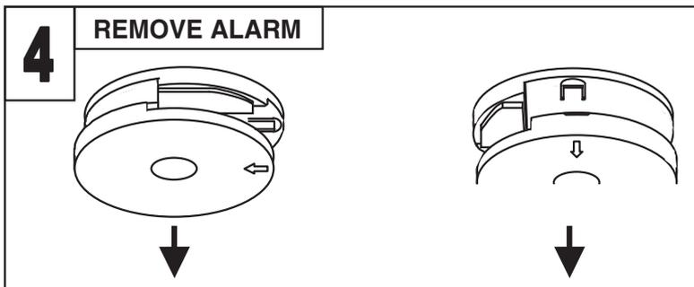
HOLD THE LOWER HALF OF THE ALARM AND REMOVE FROM THE BASE PLATE BY MOVING IT VERTICALLY DOWNWARDS, TOWARDS THE FLOOR.
