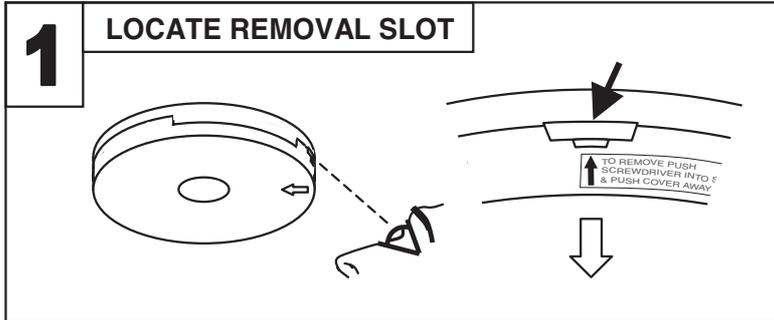
LOCATE THE ARROW ON THE FRONT FACE OF THE ALARM. THE SLOT IS LOCATED DIRECTLY ABOVE THE ARROW.
